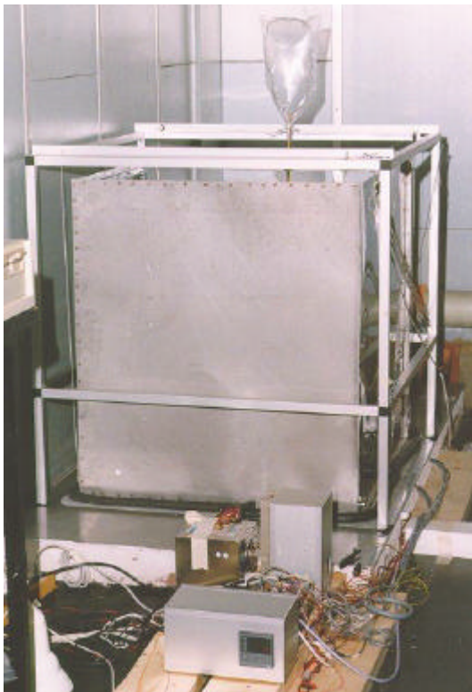
Figure 1. The climate chamber. It stands about 1 metre high. The control electronics is in the foreground.
