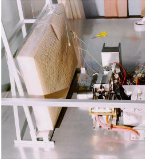
Figure 2. An experimental wall, 600 mm square, of wool insulation, mounted within the chamber. The wool is covered on the front by vapour retarding paper and sealed on the back with aluminium foil and polyethylene. Wires lead to sensors within the insulation. One of the sensors can be seen dangling in front of the wall. The water vapour flux generator is to the right with the temperature controller in a tower behind it.
