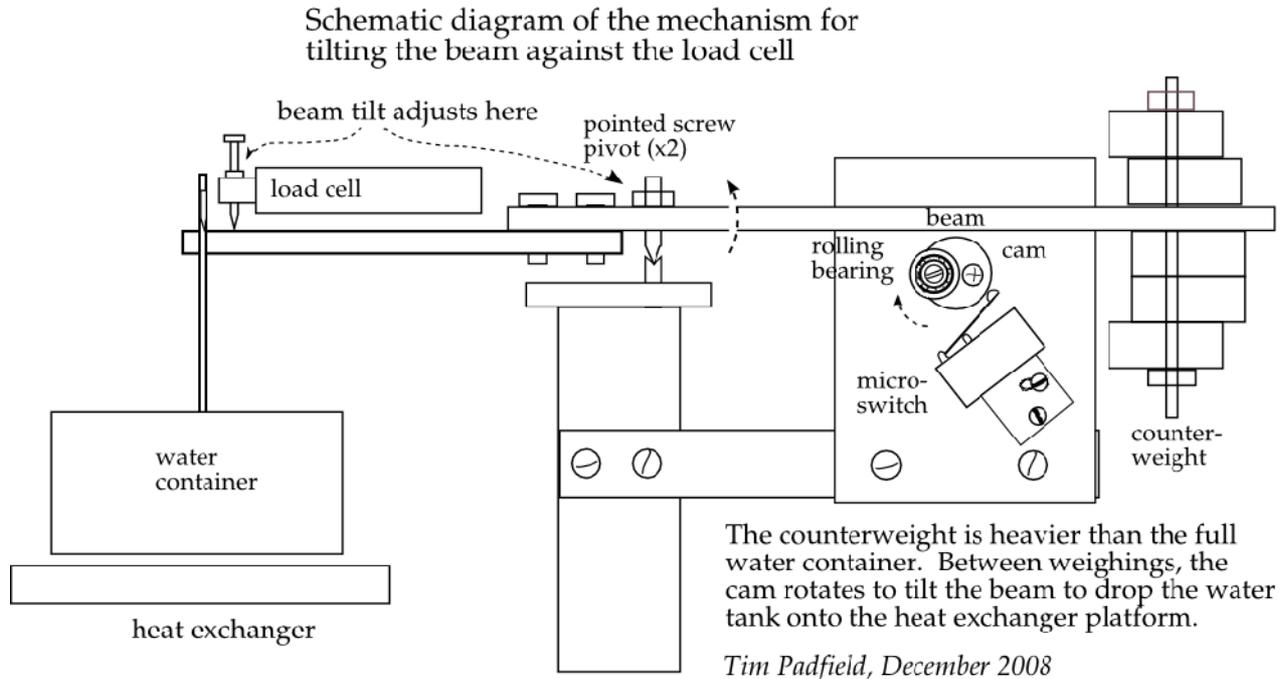
The original bending beam strain gauge has been replaced by a pivoted beam with a load cell registering the out of balance load on the beam.
